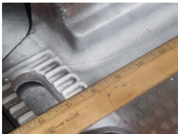
MAGNETIC PARTICLE TESTING OF RAIL FASTENER PLATES
