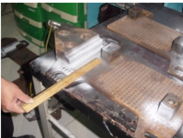
MAGNETIC PARTICLE TESTING OF RAIL FASTENER PLATES
