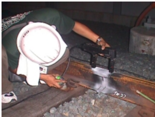
MAGNETIC PARTICLE TESTING AND ULTRASONIC TESTING OF RAIL THERMIT WELDS
